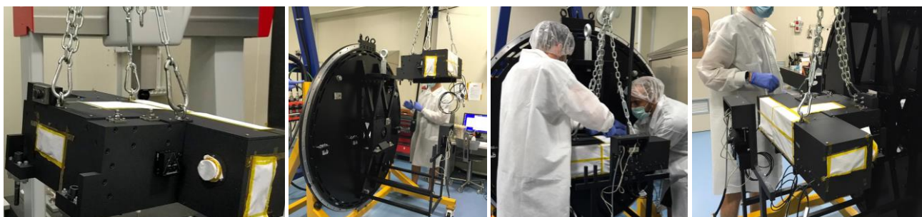
Figure 25. From left to right: CP lifted; CP in front of the IF flange; tightening of the CP KMs; CP installed.
